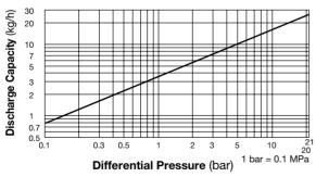
1. Differential Pressure is the difference between the inlet and outlet pressure of the trap.
